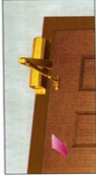
TOP JAMB INSTALLATION
